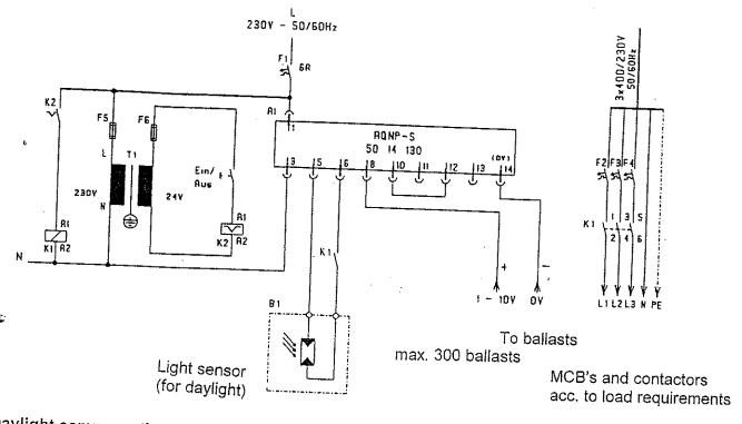
Daylight compensation control in reverse proportion to daylight AQ NP- S with ON/OFF (24V) with changeover to manual control via control panel FA
