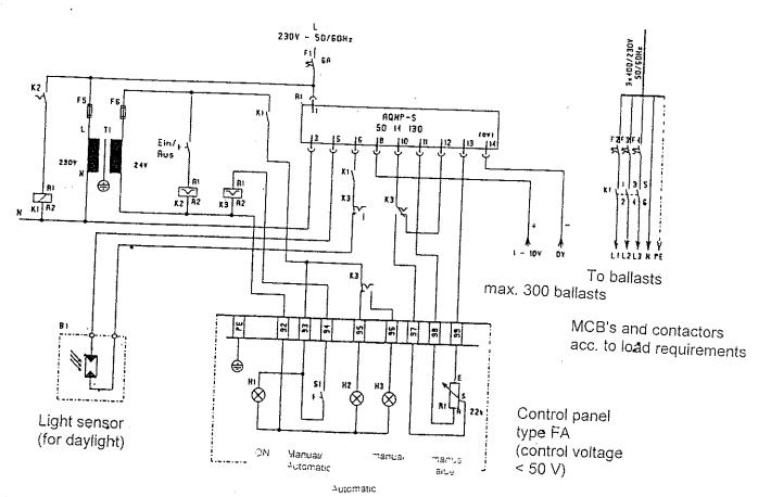
Daylight compensation control in reverse proportion to daylight AQ NP- S with changeover to a manual control with control panel FAD with ON/OFF (24V)
