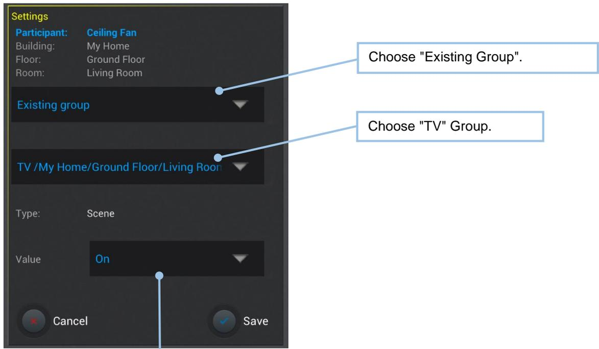
As this is an AQStation Switch, the "Value" setting allows you to decide whether the device should be turned on or off.
