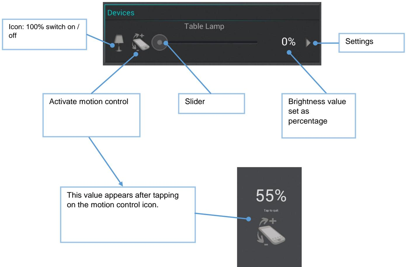
For dimmable lamps, the brightness values for the connected electrical-load devices can be set at 0 to 100 percent. Tap on the entry icon to turn the light on (100%) or off (0%). Use the slider to freely set the desired brightness value. The percentage value will appear on the right side of the slider.
